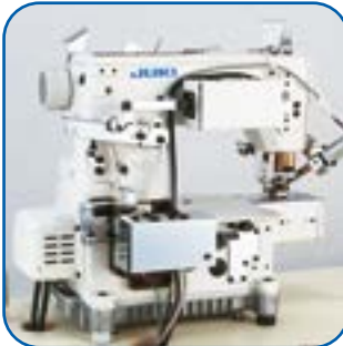
Presser lifter drive mechanism magnet Thread trimmer drive mechanism magnet
